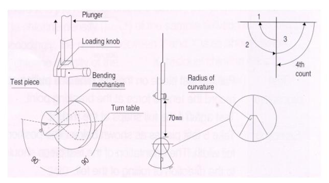
2) One 90° trip is counted as one bending. For instance, the movement shown in the diagram is counted as 4 bendings.
